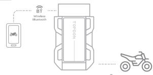
Tap **Diagnostics** on the home screen, then tap **VCl** at the top right of the screen to establish a Bluetooth connection with the unit. When connection is established, the LED light on the unit will turn solid blue.
