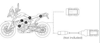
The Data Link Connector (DLC) of a motorcycle is typically located under the seat or near the engine (see the figure above).
